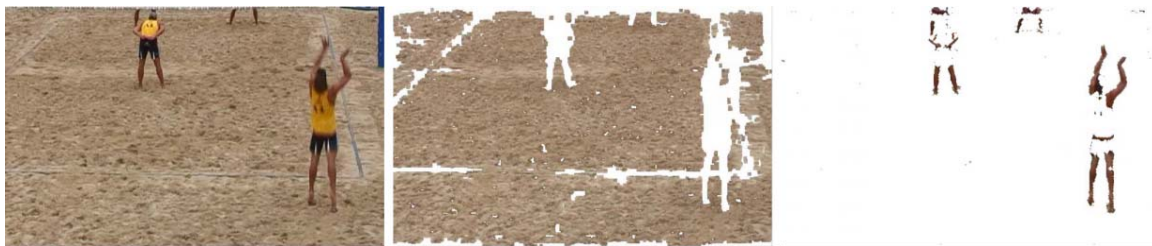
Figure 7. Left: Original input video frame. Middle: Segmented sand-colored pixel. Right: Skin segmentation can be used to create more accurate information about player positions.
